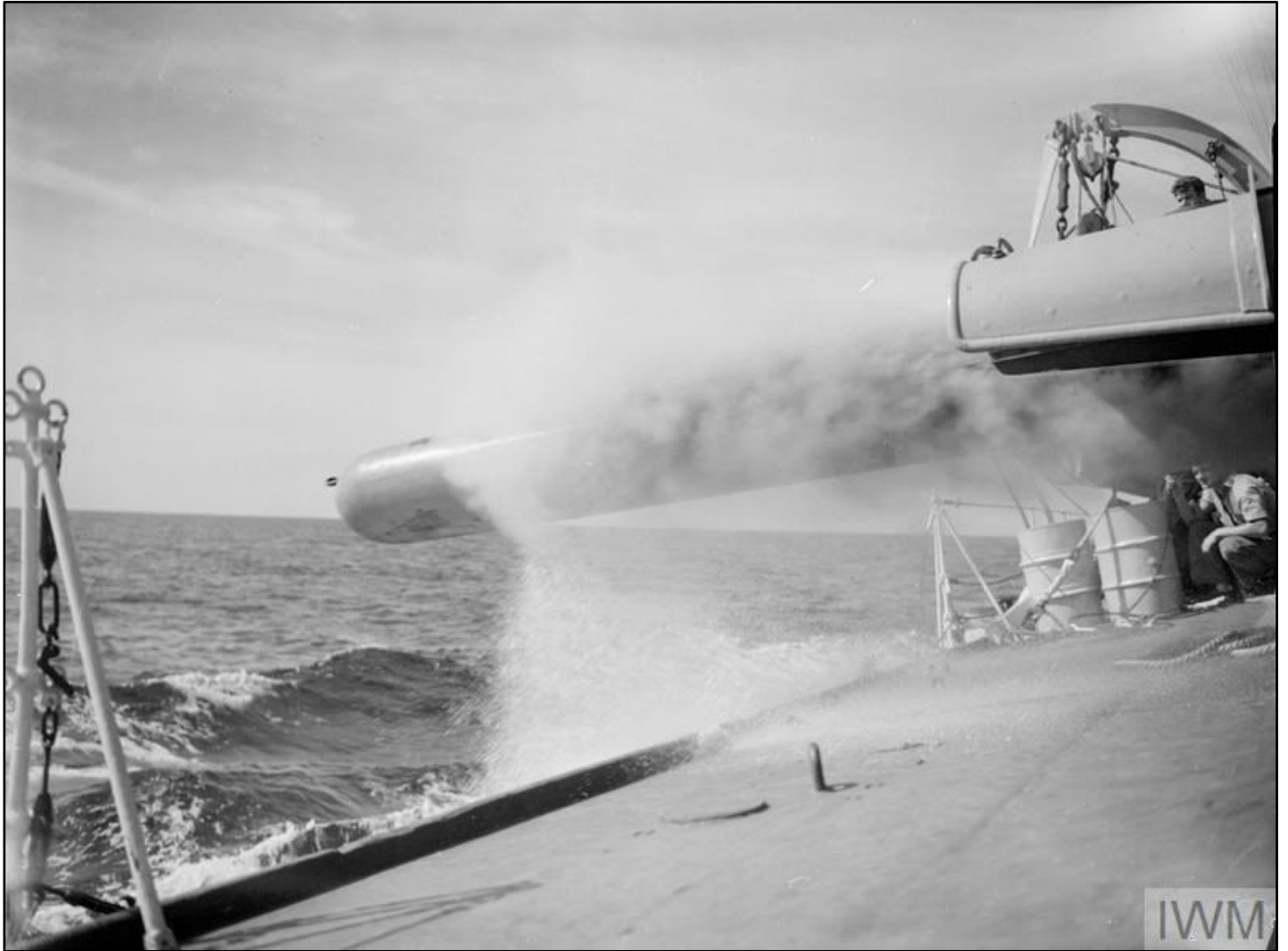
A practice torpedo leaving the tube in HMAS Warramunga enters the water at high during Commonwealth Fleet Exercises in June 1952 off the west coast of Korea. From IWM Collection (A 32240)
